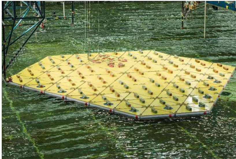
Fig. 6. Model test of the concept of a multipurpose platform with triangular floating modules.
